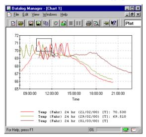
Release the mouse button, and the chart changes to an enlarged view of the area covered by the **zoom box**.
