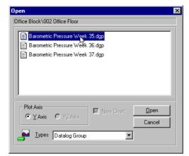
**Note:** Datalog Groups can NOT be added to an existing chart in the way that other chart types can. A Datalog Group must always be opened as a new chart. However, once a group is opened, data from other datalogs or points can be added to it.
