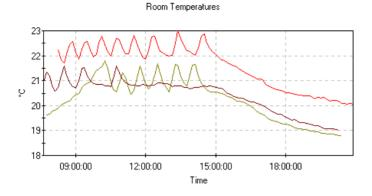
However, this kind of display can exaggerate variations in sensor readings, and make it difficult to assess the level of control present in the signal. It can be useful to set the scale of the Y axis to run from zero to the maximum plot value, to give perspective to the chart: Room Temperatures
