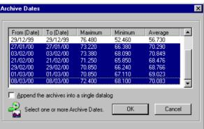
These will be inserted on a chart with each archive date as a separate plot. Only 6 plots can be displayed at once.
